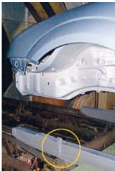
For the Ford plant in Belgium, Turck developed RFID high-temperature data carriers for reliable identification up to 210 °C – even in the furnace
