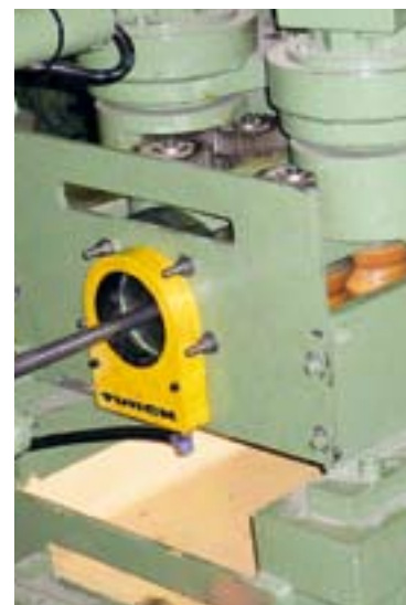
In the cold pilger rolling mills from SMS Meer, the special Turck eddy current sensor identifies the material and the diameter of a tube or pipe
