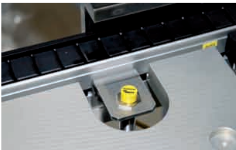
Simple mounting: All read-write heads in the Turck RFID system BL ident are fitted to standard sensor housings
