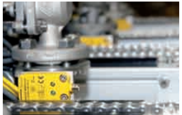
The RFID data carriers are mounted on the lower end of the workpiece carriers
