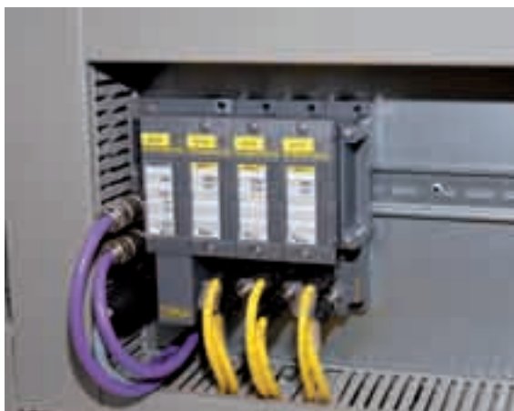
Up to four I/O modules can be connected to the BL ident gateway (left) for up to a maximum of eight read-write heads
