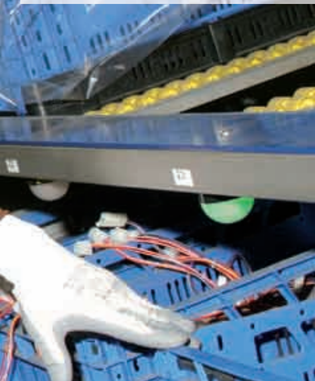
The Pick-to-Light modules from each picking station are controlled by a separate SPS – the Turck I/O System BL67 ensures reliable signal transmission
