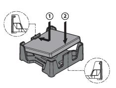
Mounting the data carrier properly in the retainer To avoid damage to the retainer, follow the instructions below. Carefully push both sides of the data carrier in the retainer until they latch (the latches are designed differently): 1. Insert data carrier
